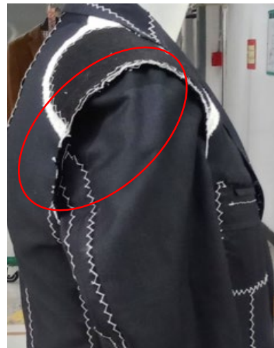
Old make you can see the lack of sleeve head which gave a messy look to the should and back of sleeve
